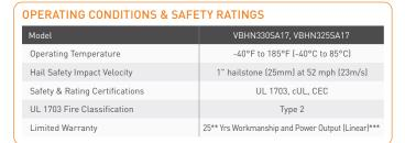
NOTE: Standard Test Conditions: Air mass 1.5: irradiance = 1000W/m<sup>2</sup>: cell temp. 25°C
